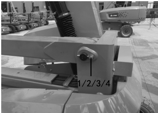
1. Pin 2. Safety pin 3. Bolt 4. Washer
