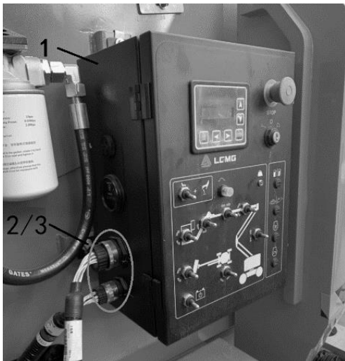
1. GCU assembly 2. Bolt 3. Washer
