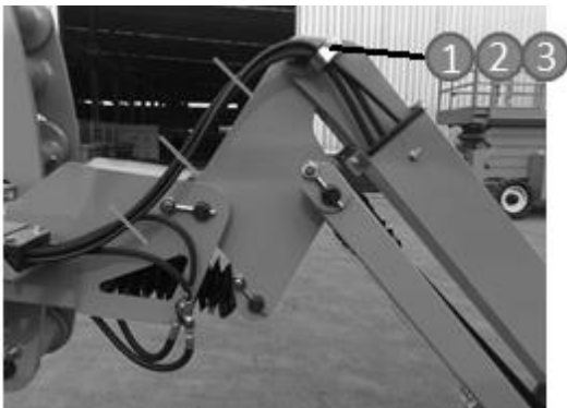
1. Pipe clamp 2. Cushion collar 3. Spacer ring
