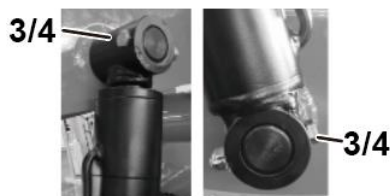
Fig. 3.35 Assembling folding jib lift cylinder
