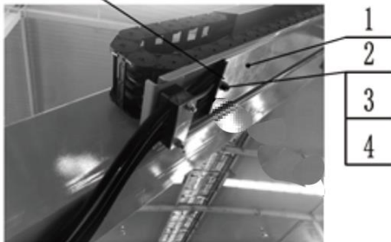
Fig. 3.20 Cover plate weldment
