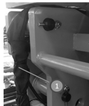
Fig. 3.34 The canvas is wound around the wire harness
