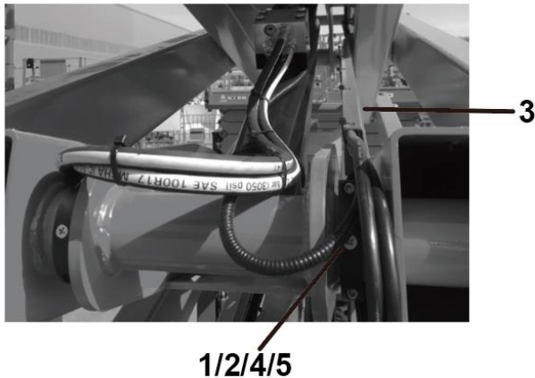
Fig. 3.27 Three-layer cable board assembly(SR4069D)
