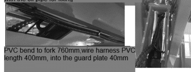
Fig. 3.31 Routing and tying the harness (SR4069D)
