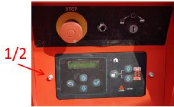
Fig. 5.21 Platform control panel
