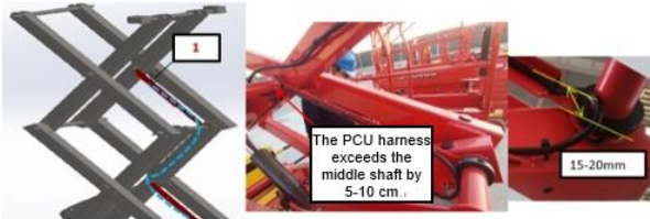
Fig. 4.29 Installation of third layer pipeline
