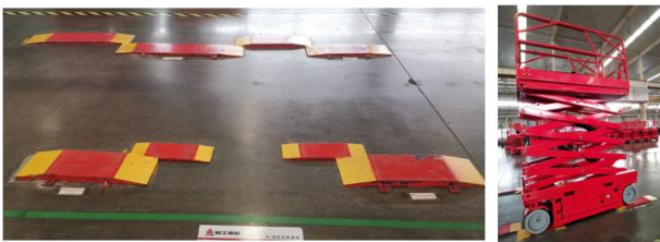
Fig. 9.14 Horizon sensor left and right inclination angle test
