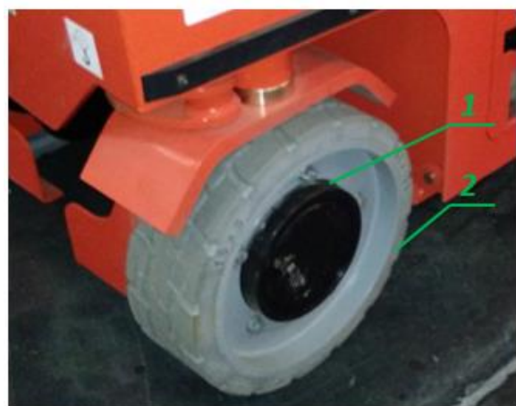
Fig. 5.31 Front Wheel Assembly (S2632 II, S2632E II, S46 II, S46E II, S4650 II, S4650E II)
